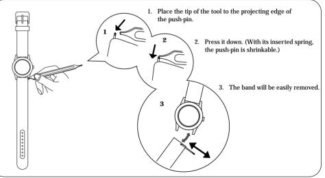
$\boldsymbol{\diamondsuit}$  The reverse procedures will be applied in order to attach the separate type band.
